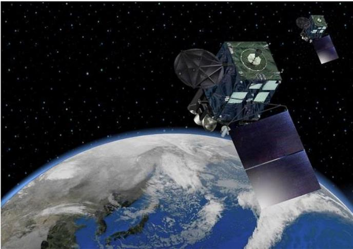
The Advanced Himawari Imager (AHI) instrument carried by both Himawari-8 and -9 records more data than previous geostationary meteorological satellites—16 channels, including three visible wavelength bands (red, green and blue) to create ‘true-colour’ images of the Earth. Different channels give us greater insights into different characteristics of the atmosphere.
